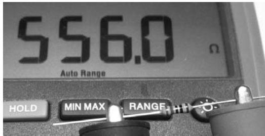
Figure 3-4: Multimeter measuring a 560-ohm 1 percent tolerance resistor
